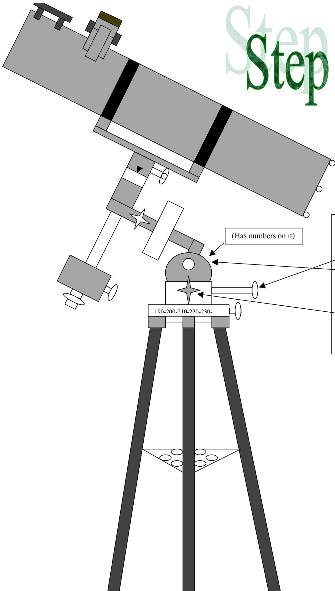
Next, you will need to elevate the telescope up to the North Star. Do this by turning the **Latitude Adjustment Knob** to the number on the Star Atlas that corresponds to your location. Looking through the eyepiece, find the North Star then tighten the **Latitude Lock Knob**. Note: when this is done you will not have to touch either of these knobs again for the rest of the night.
