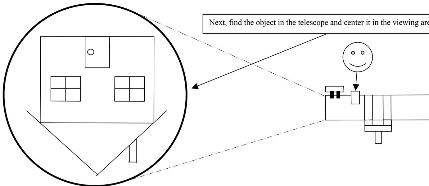
Finally, get the object centered in the finderscope. If the finderscope is not the crosshair type but instead the dot kind, get the dot directly in the middle of the object then tighten the finderscope best as possible. Note: The finderscope just like the telescope turns the image upside down also.
