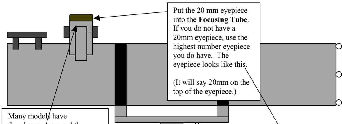
Many models have thumbscrews around the **Focusing Tube** to tighten the eyepiece down. Even if there aren't any, they are probably not needed.
