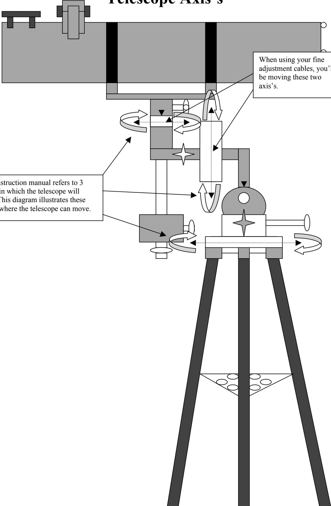
When using your fine adjustment cables, you'll be moving these two axis's.
